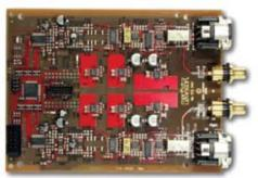
DAC PCB on six-layer, high-speed Nelco® N4000-13 SI laminate. The intricate, mirror-image PCB design shows the care that was taken to place every component and trace.
